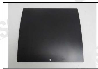
Photo A: Appearance of the sample (Hardness by pencil)
